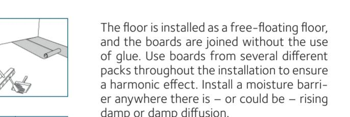
The floor is installed as a free-floating floor, and the boards are joined without the use of glue. Use boards from several different packs throughout the installation to ensure a harmonic effect. Install a moisture barrier anywhere there is – or could be – rising damp or damp diffusion.
